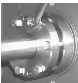
Tighten Capscrews – More Than One Rotating Sequence
